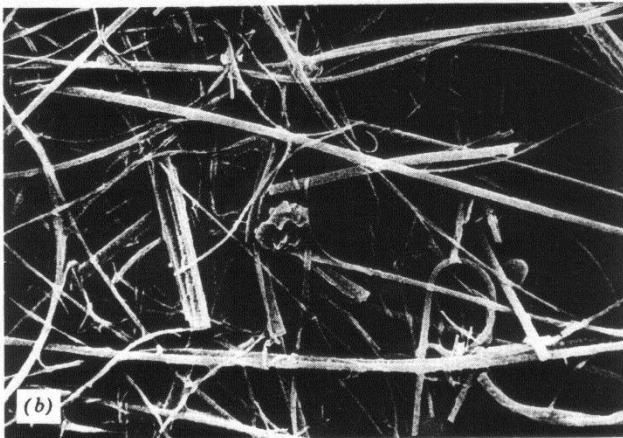
9.1 Scanning electron microscope photograph of a high-efficiency glass fiber matification of (a) 4150 \times and (b) 800 \times .
